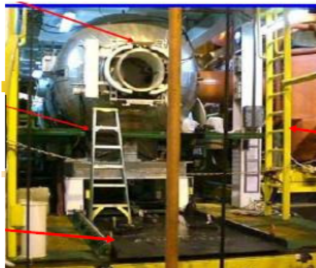
Saturation chamber from which diver fell
