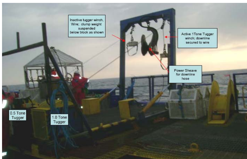
A-frame with tugger winch, snatch block and powered sheave arrangement
