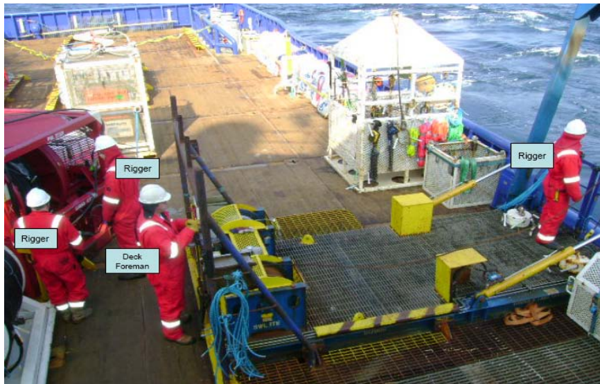
Position of deck crew during downline/tugger wire recovery
