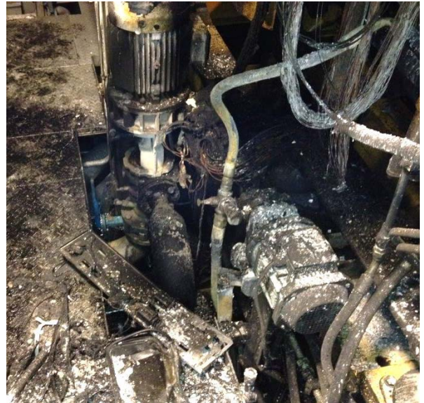
Figures 7 and 8: showing damage to the engine room following the fire
