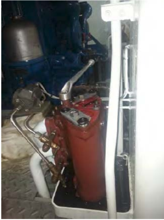
Figure 1: Typical fuel filter of the sort that failed
