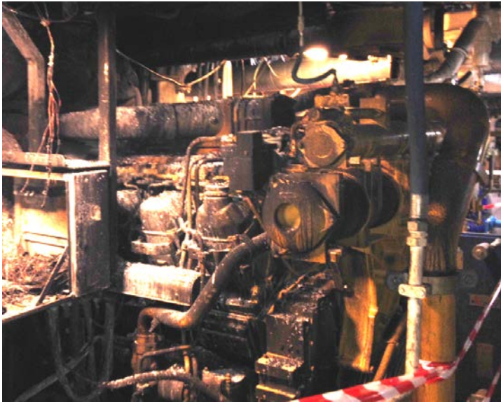
Figures 7 and 8: showing damage to the engine room following the fire
