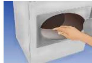
**Clean the lint out of the inside of the dryer regularly** – your dryer needs to be opened up and vacuumed out periodically.
