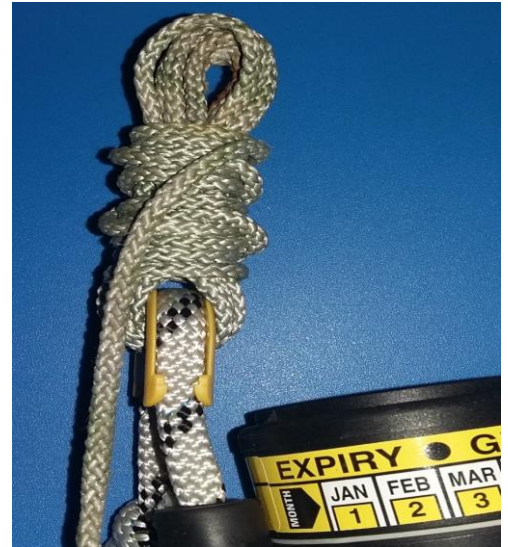
Lashing tied too tight where usually connected to Senhouse slip
