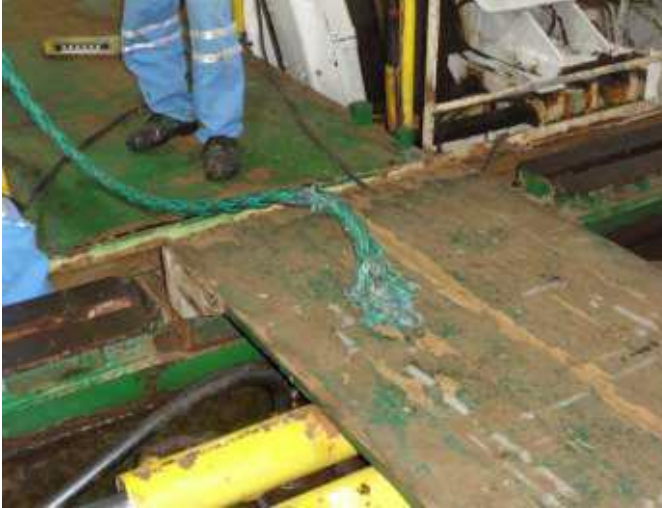
Parted rope on deck
