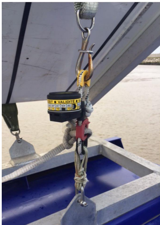
Correctly stowed HRU on life raft
