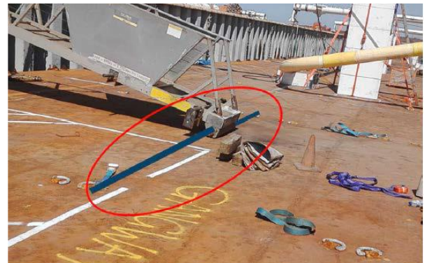
Gangway secured at low end (roller end) using a cargo strap.
