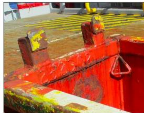
Basket stacking pins snagged on inside of protective rail
