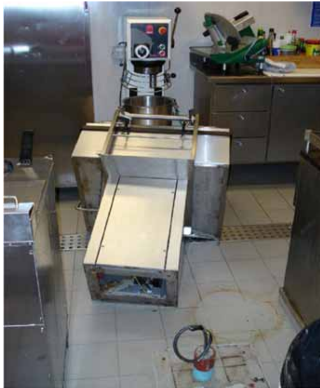
Grill fryer toppled over on floor of galley
