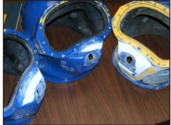
The unauthorized paint job on these helmets concealed repairs performed with sub-standard materials.
