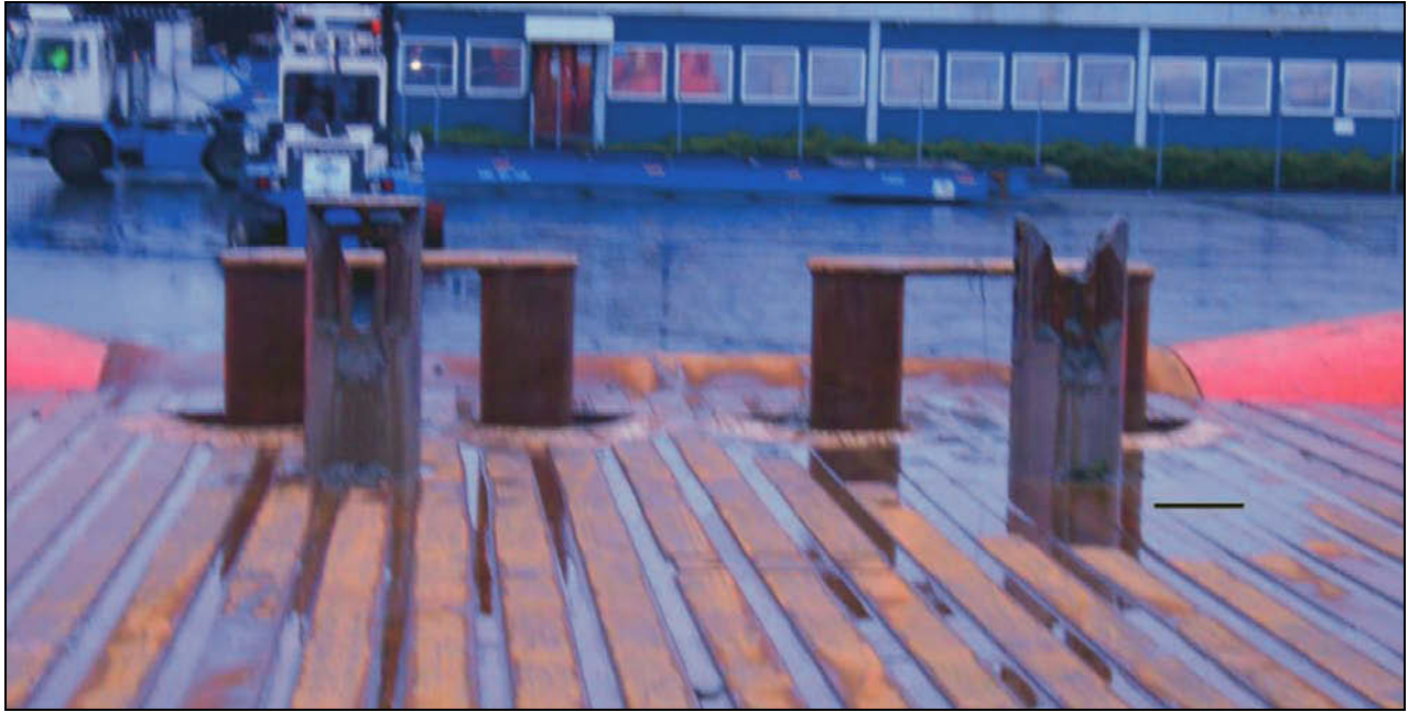
Figure 5.9 Photograph of shark-jaws and towing-pins
