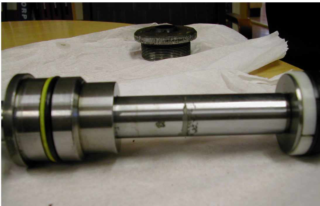
Picture 3. Piston rod has clearly a damaged area.
