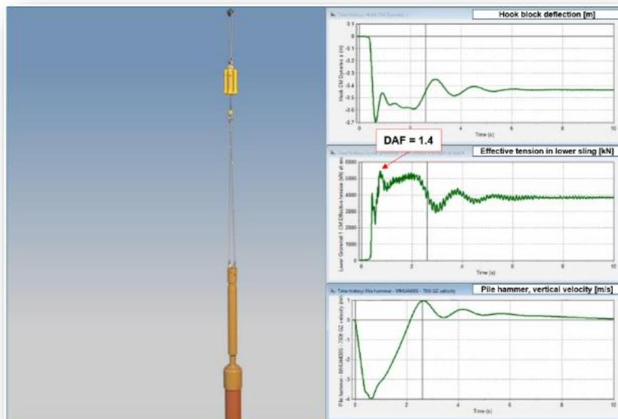
Figure 28 – Pile run with damping
