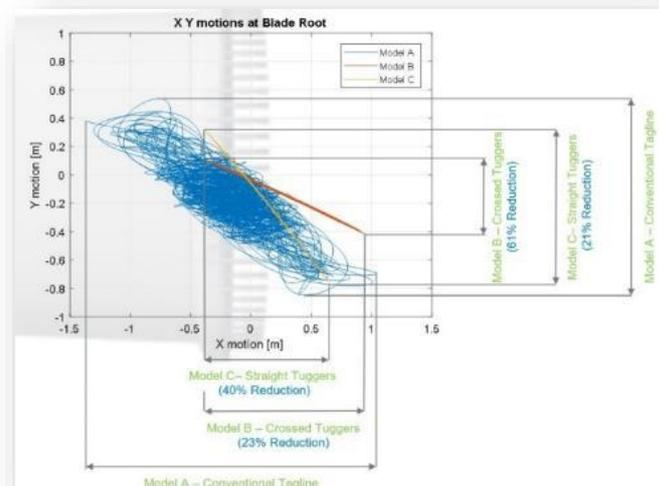
Figure 38 – Reduction in blade root motions
