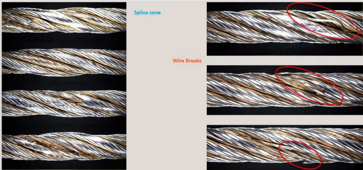
Figure 45 – Defect identification
