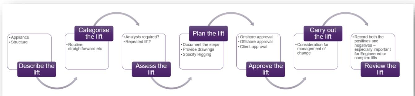
Figure 7 – Lift Plan Process
