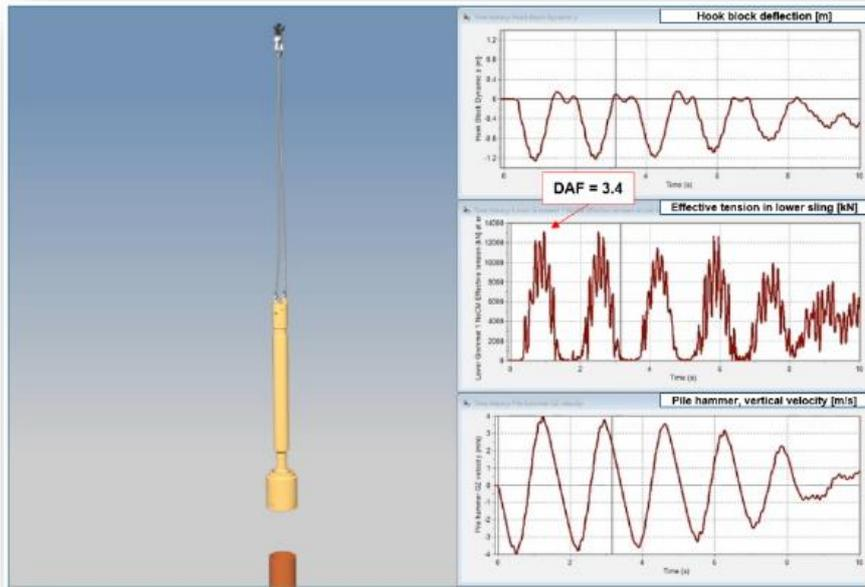
Figure 27 – Pile run; no damping
