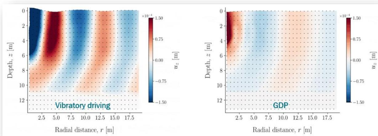
Figure 55 – Vibratory Driving Vs GDP Shaker
