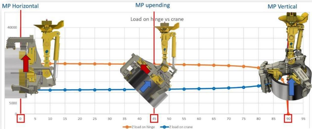
Figure 25 – Tool position during upending
