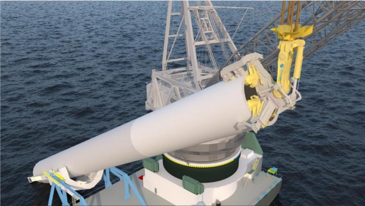
Figure 23 – Monopile upending and lifting tool
