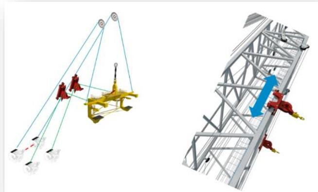
Figure 37 – Travelling load stabilising system
