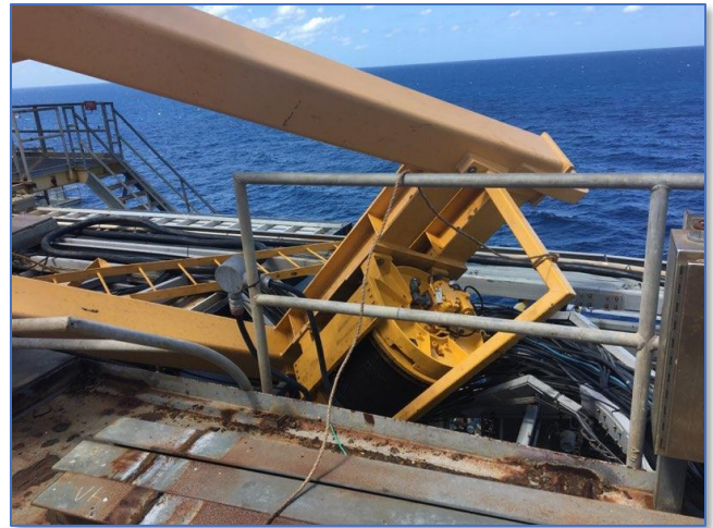
Figure 2. Gantry Contacting and Damaging the Cable Tray and Bending the Main Deck Handrail
