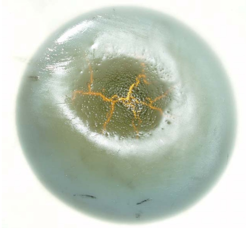
Figure 22a: HDPE panel after water test (view from liquid side). The failure mechanism is pitting to produce holes a few hundred micron across. The characteristic leakage rate is of order 1 g/s
