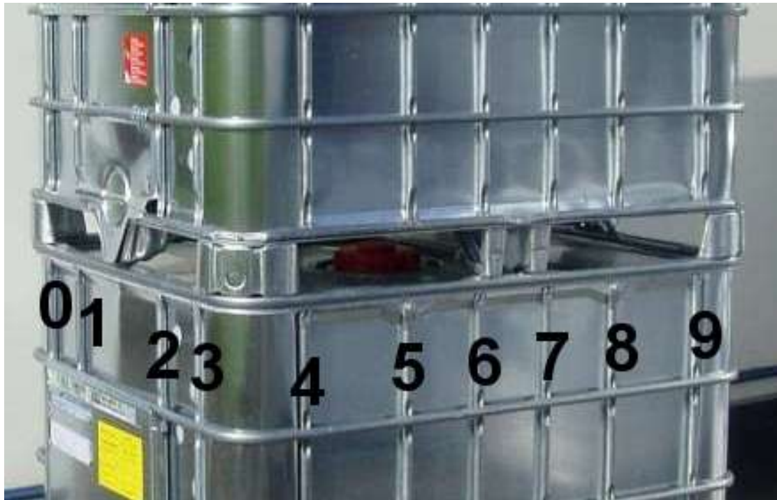
Figure 8: Locations of thermocouples recording steel tube temperature
