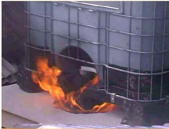
Figure 20: Fire in an IBC containing an industrial lubricant (flashpoint 75°C)
