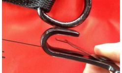
The issue is the spring-loaded tab in the snaphook on the waist belt affecting **some** REVERE lifejacket models 198 RT and 160 RT. The tab has been found to be too long for both the thick or thin design,. When the D-ring of the main waist belt is "hooked," the length of the tab prevents it from snapping closed. With the hook remaining open, the D-ring is not fully secured. (top photograph) The spring-loaded tab may also lose its resiliency. (bottom photograph)
