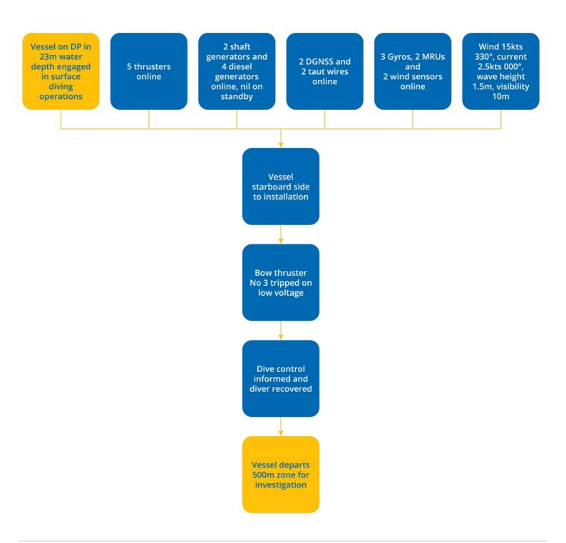
The seat for the stop solenoid on the port main engine was damaged causing a slight air leak past it, this acting on the stop cylinder piston caused a reduction in main engine rpm. The reduction in rpm caused a low voltage alarm followed by breaker trip and low frequency alarm. Power was lost to bow thruster No.3 due to a breaker trip on the switchboard, the port azimuth thruster was not affected as the clutch out rpm was not reached.
