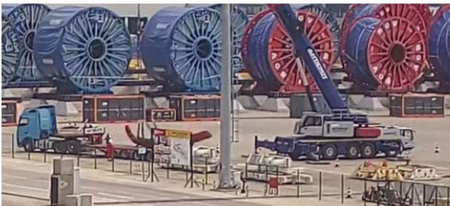
CCTV footage showing the cradle insert falling from trailer
