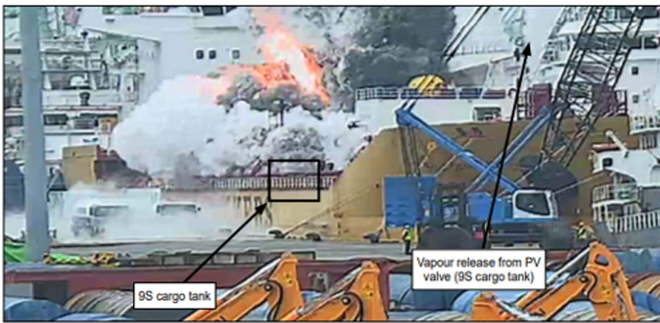
Figure 1: Tank rupture and ignition of released vapour
