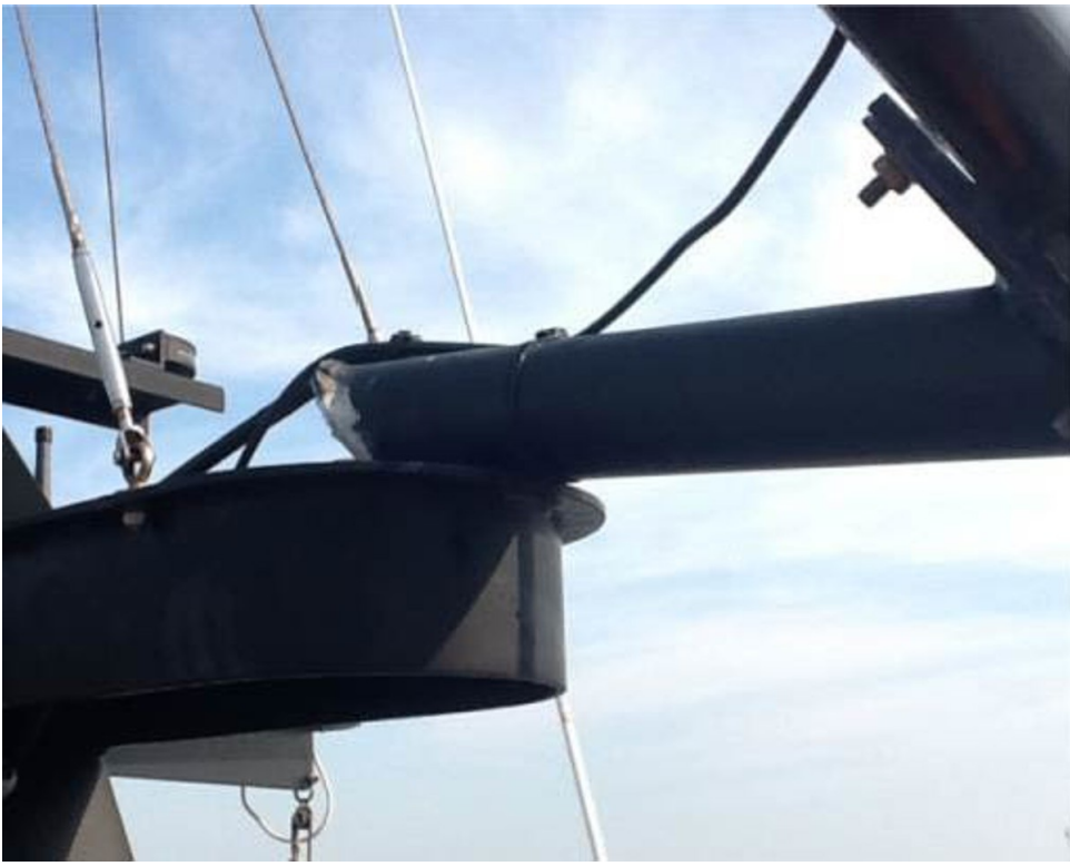
Mast damage following the first incident
