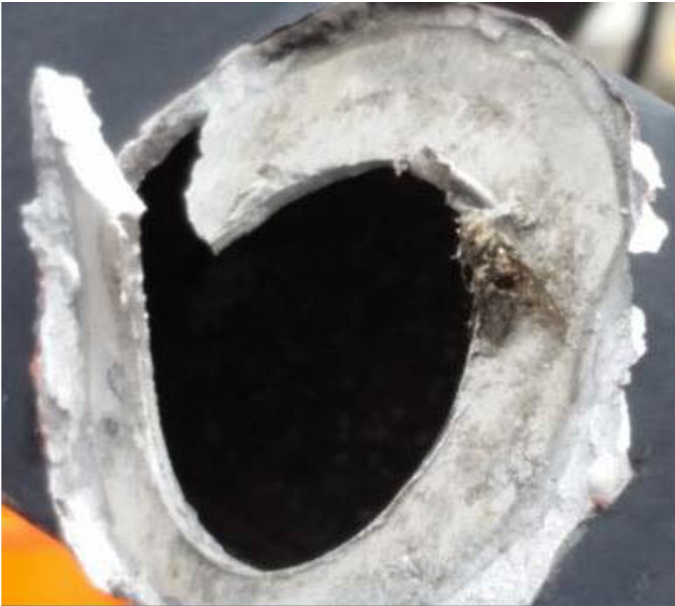
Mast damage following the second incident
