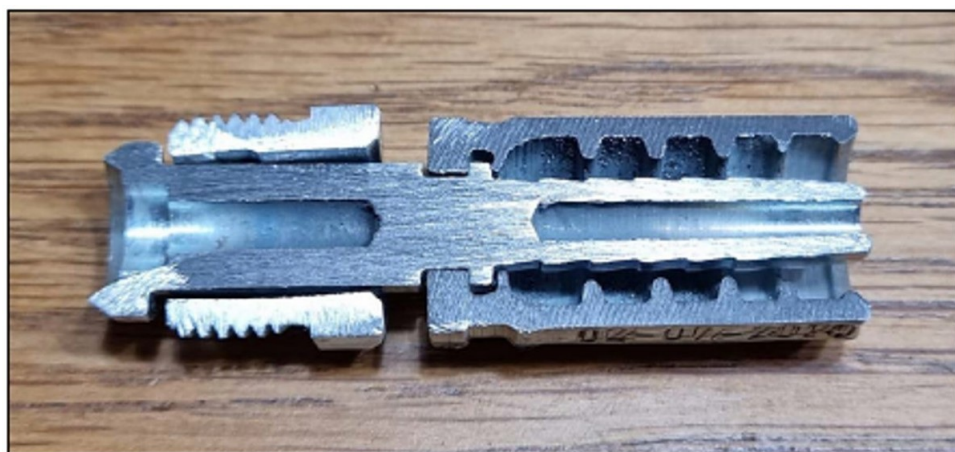
Section through blocked CO 2 pilot hose coupling showing incomplete bore through the stem
