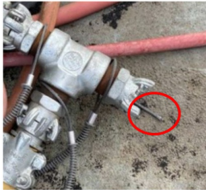
Figure 2 - Broken whip check from the incident.
