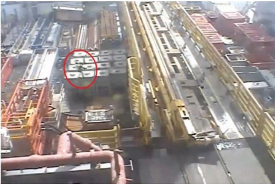
Figure 2: Worker lifted with load after becoming entangled
