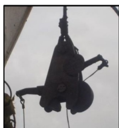
Image 1 - Davit Hook failed, releasing and dropping the workboat (vessel 1)
