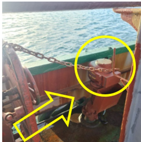
Hatch cover held by chain and hooked to a hose support
