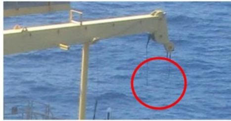
Figure 2 – Crane missing main block and auxiliary ball
